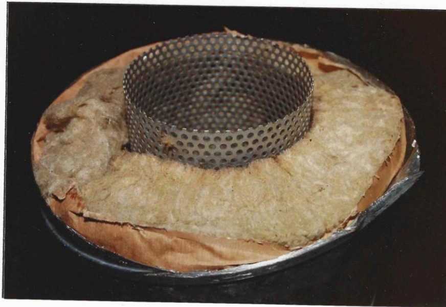
Fig. 4.1 (c) The silencer. Notice the structure of the lining.
